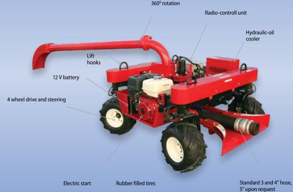
The Line Dragon machines, weighing about 410 kg and 450 kg, are driven on wide rubber filled tires, which minimize the evenly spread weight per cm<sup>2</sup>. The 'placer' is attached to the end of the delivery line (hose) and places concrete where you need it, while the 'dragger' is placed 6-12 meters before the "placer", keeping the excess line out of the pouring area.
